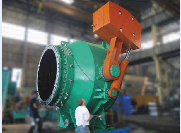
Functional testing of specially developed double-sealing Spherical valve DN2100 PN18 that is installed at the turbine inlet in HPP Lajanuri, Georgia. For this project VAPTECH delivered also bypass system, hydraulic pressure unit and control system.
