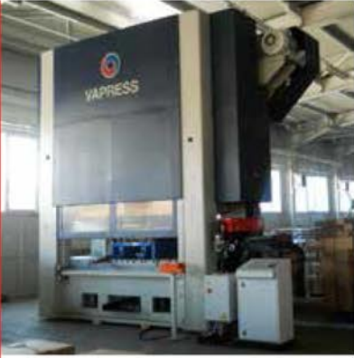
Automated press line based on 315 tons mechanical H-frame press • Berevoesti, Romania
