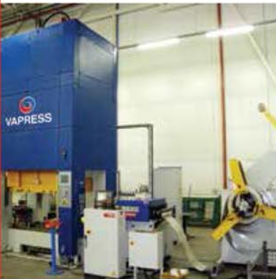
Automated press line based on 315 tons hydraulic H-frame press • Tosno, Russia
