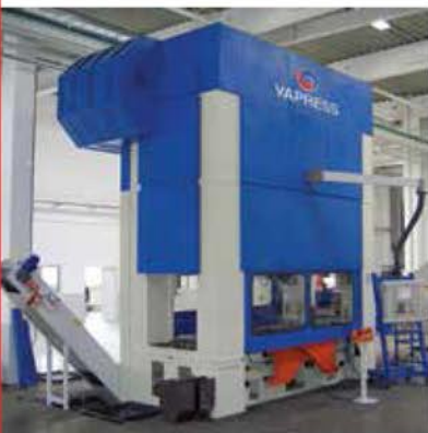
Automated press line based on 630 tons mechanical H-frame press • Erfurt, Germany
